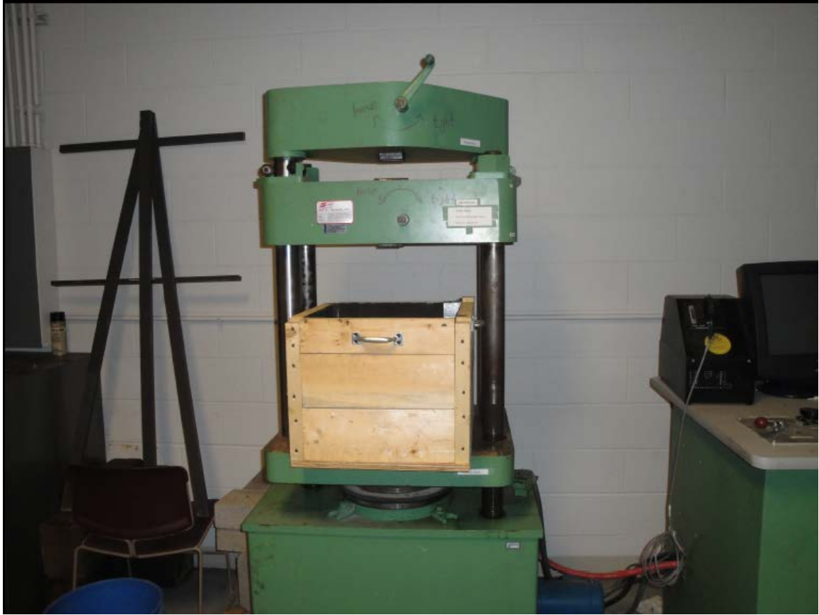
Figure C.2 Small test box.
