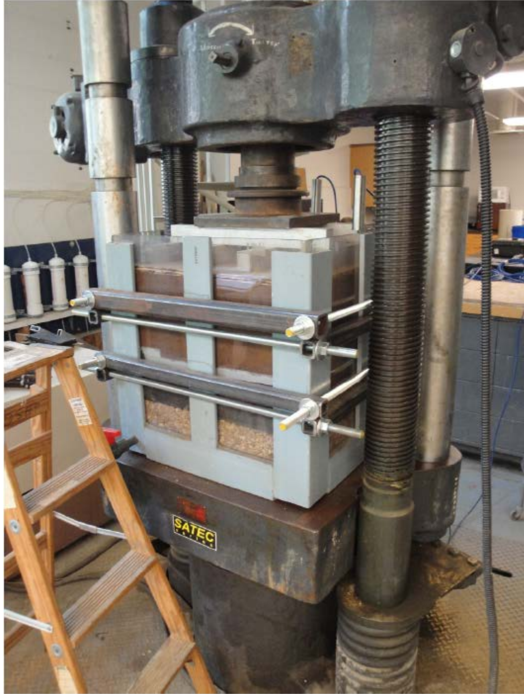
Figure C.3 Large box test setup (Huff, 2010).
